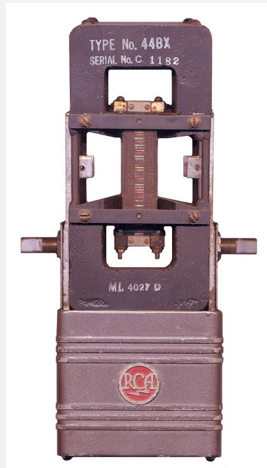
Shown here are two ribbon microphone pickup “motors” or elements. In both cases you can see the thin foil suspended within a strong magnetic field. The entire mechanical structure has to be free of any resonating or loose mechanical parts. Usually it is mounted on an internal shock-mounting system to decouple any floor, stand, or case vibrations.
