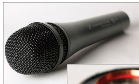
This is a dynamic Sennheiser MD835 - mic. (above) The ribbony thing (Right) is the voice coil and diaphragm from a dynamic mic - macro shot - to show the wire coil. It's about a 1/10 human hair thickness,
