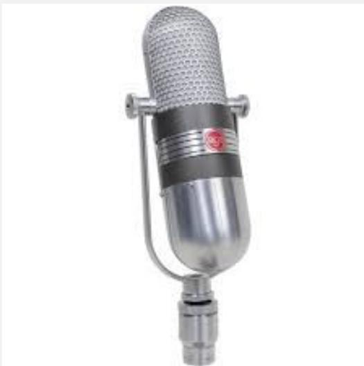
Here is the RCA 77 DX. It's one of the most identifiable “radio microphones” in studio use. These mics are expensive and durable as long they are used indoors. If they are used outside, the duralumin corrodes from the moisture.
