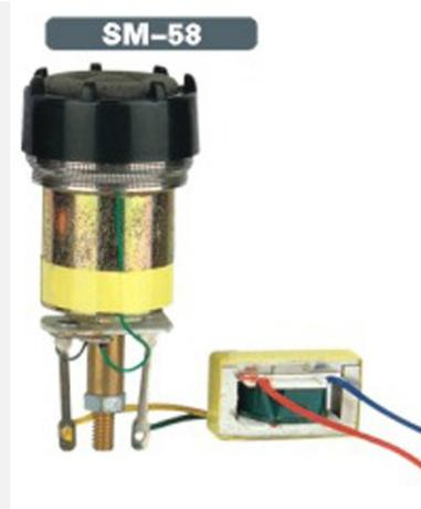
Shown here are three popular dynamic microphones manufactured by Shure Co. Shown above are the dynamic microphone, element and matching transformer to a popular a hand-held microphone known as SM 58. Above right is the little transformer that steps up the 10 ohm (or so) capsule impedance to 150 ohms. 150 ohms is the typical input impedance of PA systems and recording devices. These mics are rugged and work for decades with a little care.
